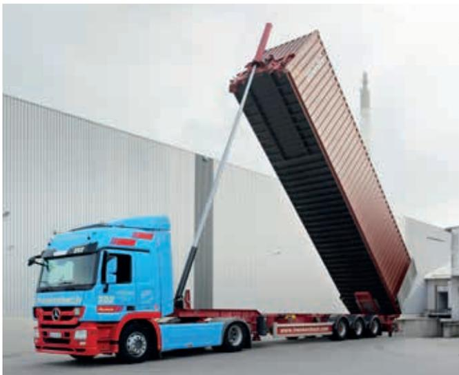
**Figure 1** 40-ft container in fully tilted position (Courtesy of Frankenbach Container Service GmbH, Mainz-Kastel, Germany)
