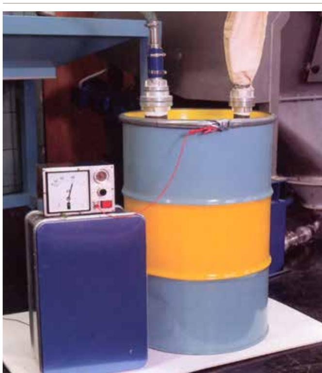
**Figure 22** Filling an insulated metal drum
