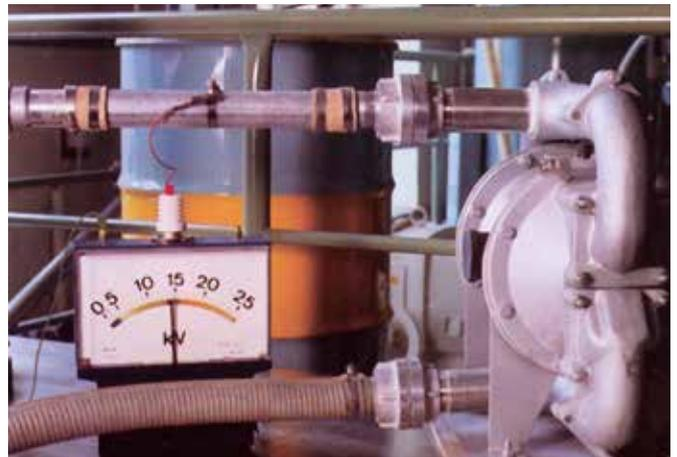
Figure 21 Part of pipe insulated from conveying system
