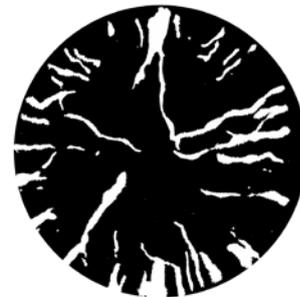
**Figure 17** Photo of a cone discharge inside a silo: top view of bed of material, with central filling port
